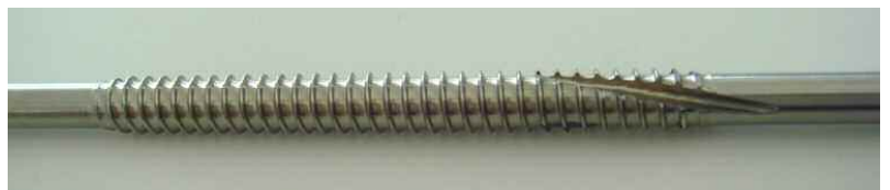
Example of the production of a transfixing pin made on our Maier ML20F:
