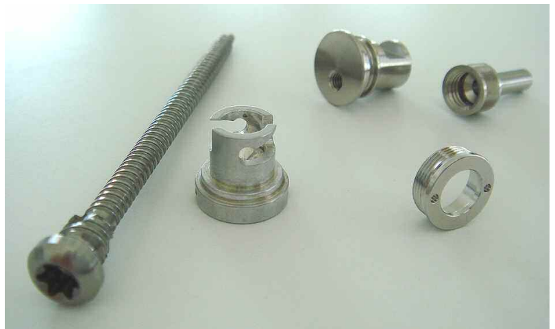
Some recent examples of parts made on our DECO 2000/13: a bone screw in titanium with double-started multilevel whirled thread with self-cutting ability and hexagonal inner torx, an aluminium turned part with bayonet drilling, three separate turned parts made of rustfree chrome steel with exact fit and millings, partially with high-frequency spindles.
